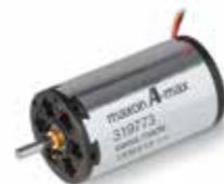
maxon A-max 26 Ø 26 mm, graphite brushes, 7 W
