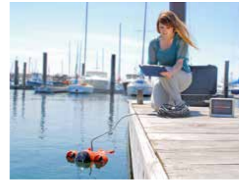
The HydroView remotely operated vehicle operates from 10 volts DC for up to three hours dependent on how it is used. It can be controlled using an iPad or PC laptop.
