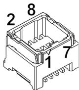
Figure 3-20 Encoder connector X5
