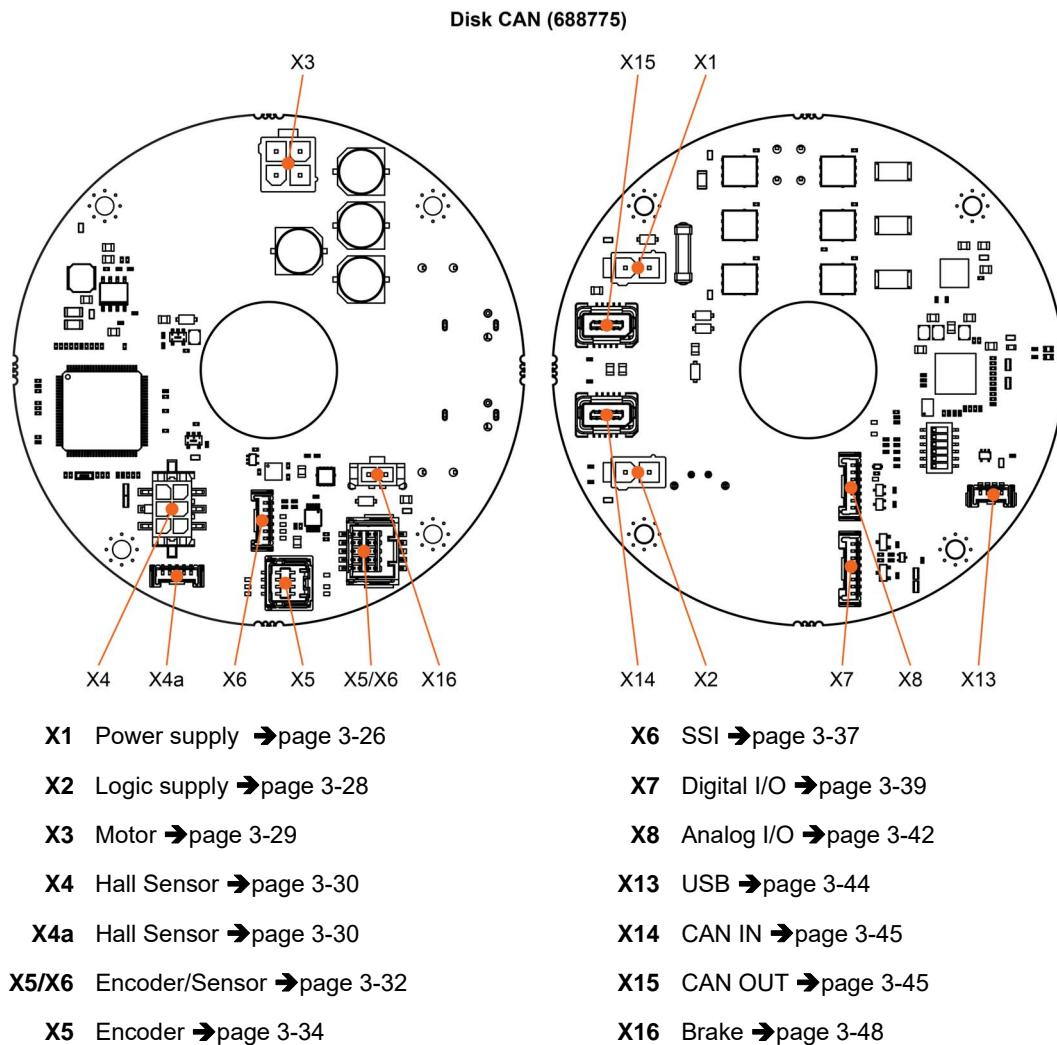
Figure 3-8     EPOS4 Disk 60/12 CAN (688775) – Connectors
