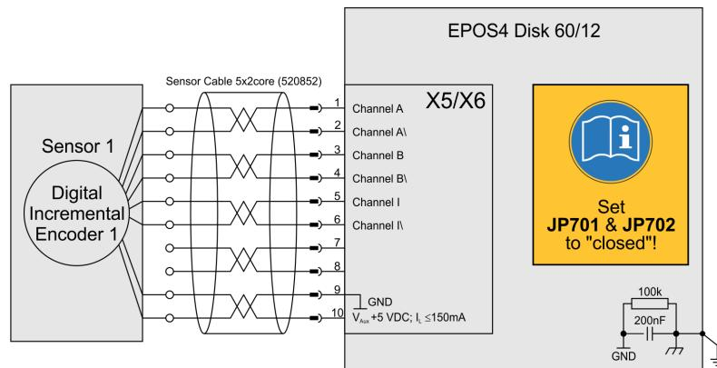
Figure 4-51 Digital incremental encoder (Sensor 1) on X5/X6
