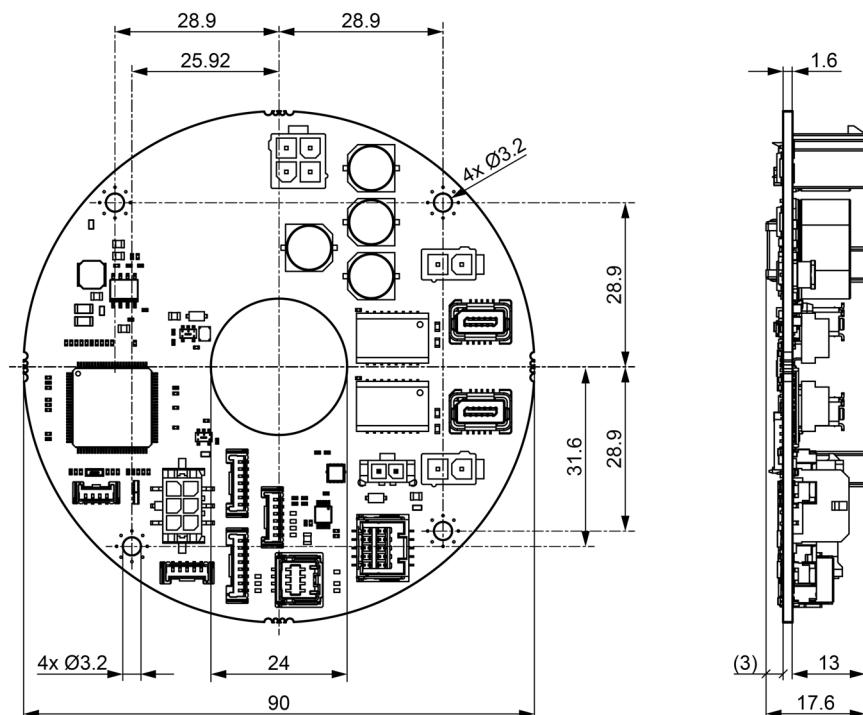
Figure 2-7 EPOS4 Disk 60/12 EtherCAT SSC (709862) – Dimensional drawing [mm]
