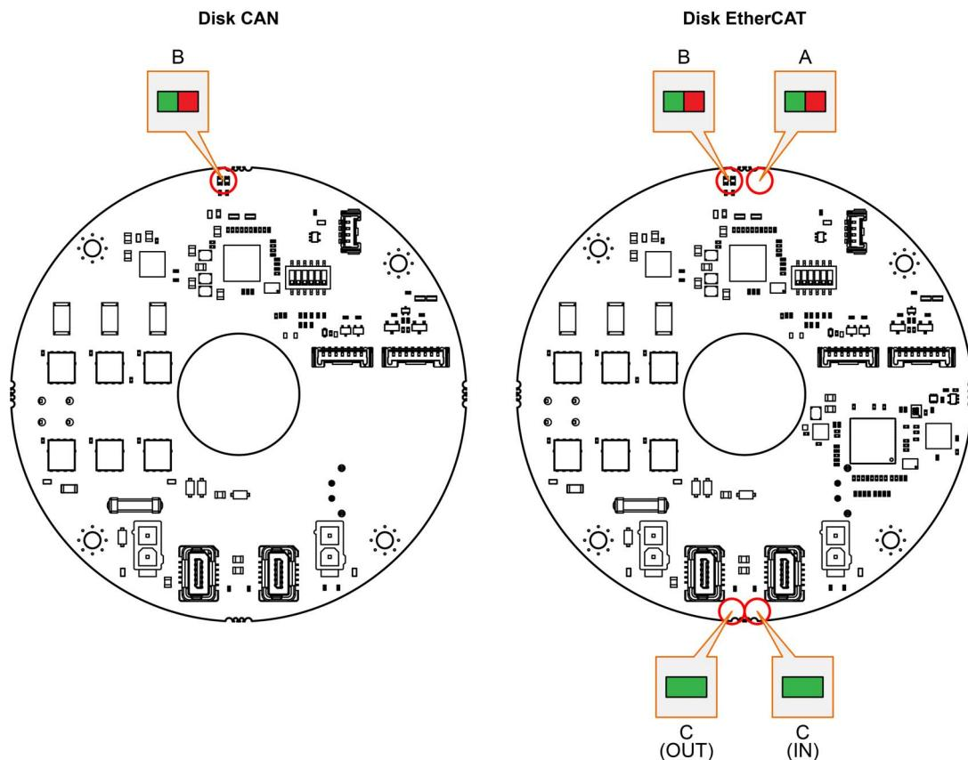
Figure 3-40 LEDs – Location
