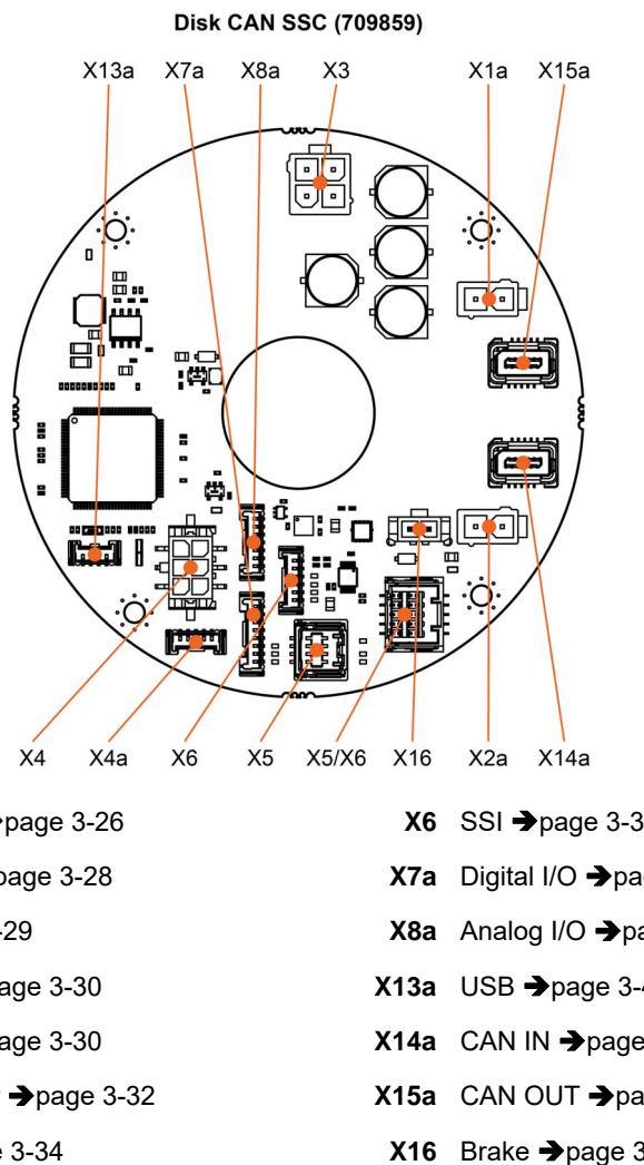
Figure 3-9      EPOS4 Disk 60/12 CAN SSC (709859) – Connectors
