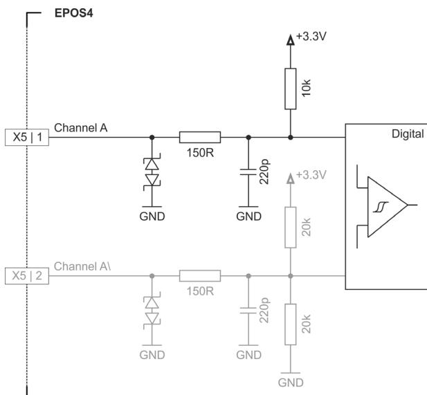
Figure 3-22 Digital incremental encoder input circuit Ch A "single-ended" (analogously valid for Ch B, Ch I, and X5/X6)
