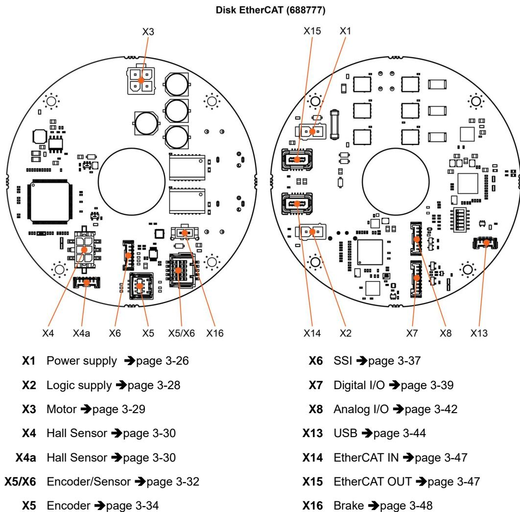
Figure 3-10 EPOS4 Disk 60/12 EtherCAT (688777) – Connectors
