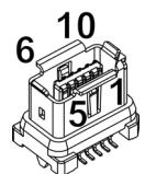
Figure 3-36 EtherCAT IN connector X14 or X14a / EtherCAT OUT connector X15 or X15a
