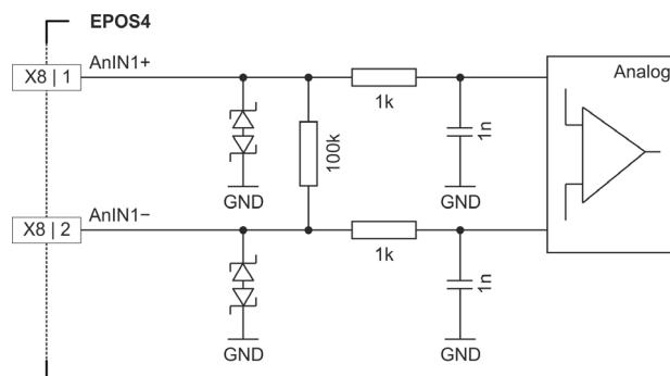
Figure 3-32 AnIN1 circuit (analogously valid for AnIN2 and X8a)
