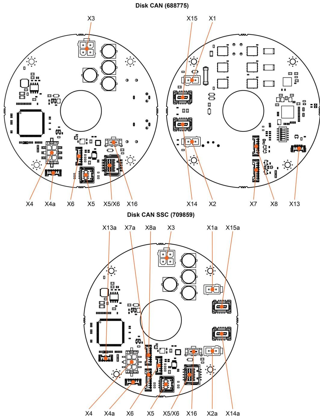
Figure 4-41 Interfaces – Designations and locations on Disk CAN
