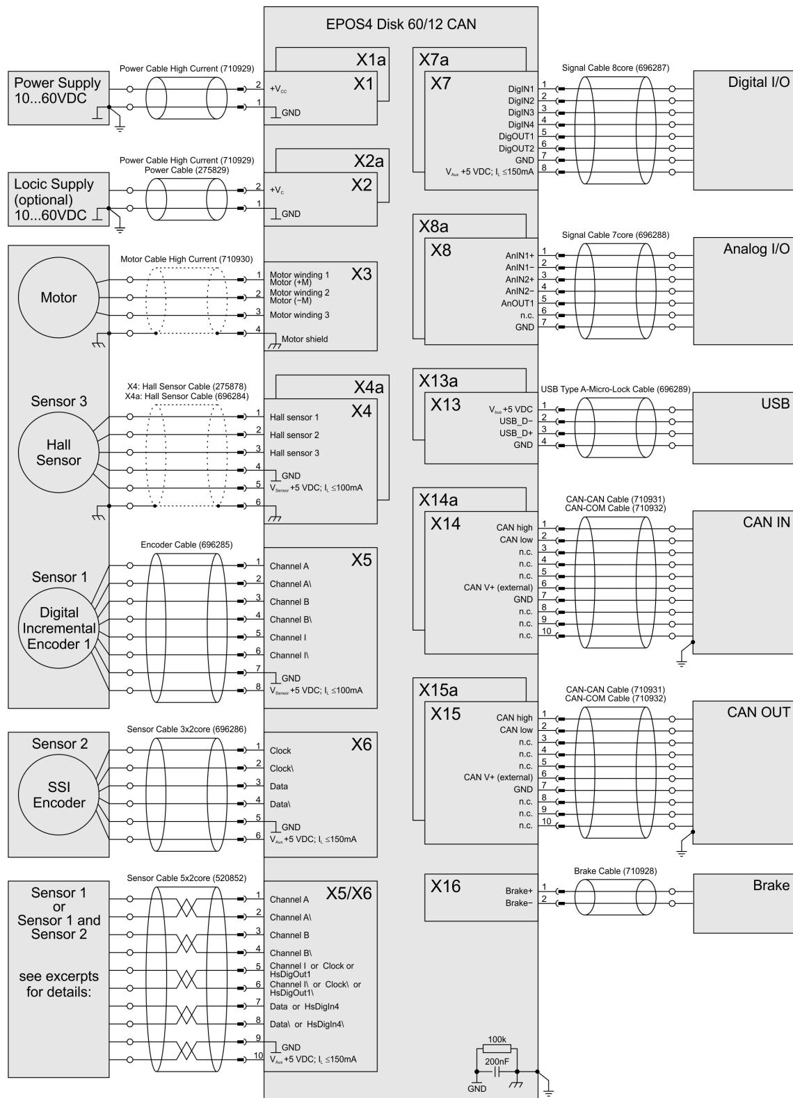
Figure 4-43 EPOS4 Disk 60/12 CAN – Main wiring diagram
