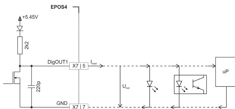
Figure 3-30 DigOUT1 "source" (analogously valid for DigOUT2 and X7a)
