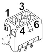
Figure 3-15 Hall sensor connector X4
