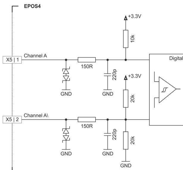
Figure 3-21 Digital incremental encoder input circuit Ch A "differential" (analogously valid for Ch B, Ch I, and X5/X6)
