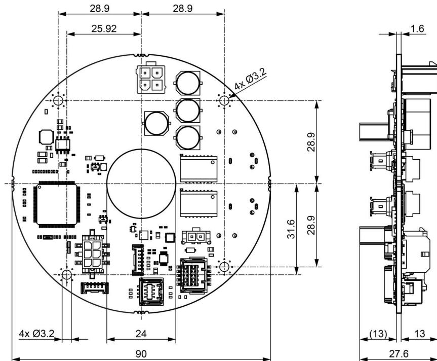
Figure 2-6 EPOS4 Disk 60/12 EtherCAT (688777) – Dimensional drawing [mm]
